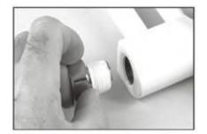
2. Tighten the nut (on the tail thread) using an appropriate tool, usually an Allen key.
